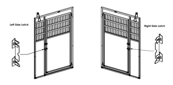
Latch Assembly can be ordered as either left or right
