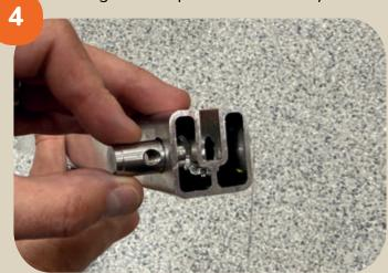
Barrel nuts insert into crossbars.
